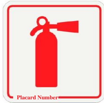
Figure 4-2. Example of a placard for safety and emergency equipment (courtesy of Airbus)
