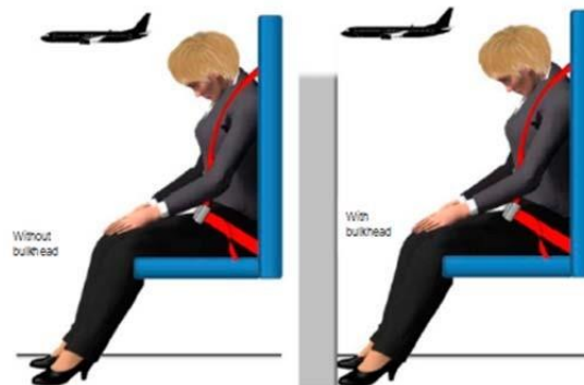
Figure 6-1. Brace position in forward-facing cabin crew seats, without and with a bulkhead
