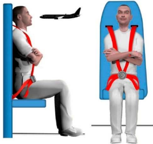
Figure 6-2. Brace position in rearward-facing cabin crew seats, without and with a bulkhead
