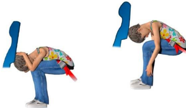
Figure 6-3. Brace positions in forward-facing passenger seats equipped with a lap strap seat belt only
